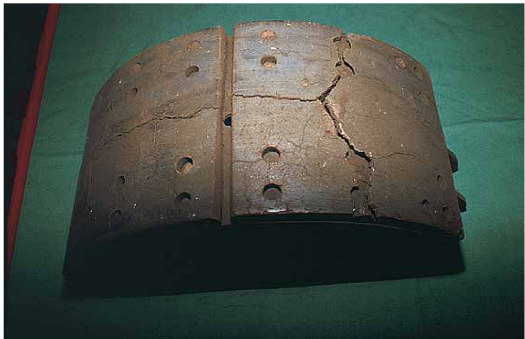
Cracked linings likely were loose on the shoe. This is caused by a shoe that's out of arc, rust buildup on the shoe surface or improper riveting.
